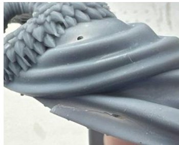
Figure 4 – Delamination of the part
