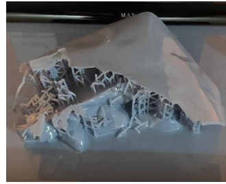
Figure 3 – Detachment from the platform during printing
