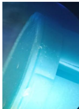
Figure 2 – Delamination between base layers and regular layers
