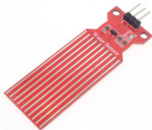
Fig.8. Module for determining the fuel level [15]
