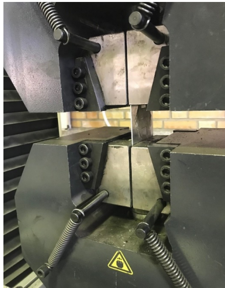
Figure 2: Positioning the Sample in the Load-cell
