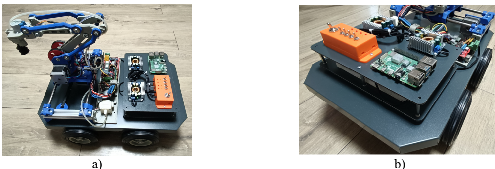
a) total view of MRP; b) MRP control system.
