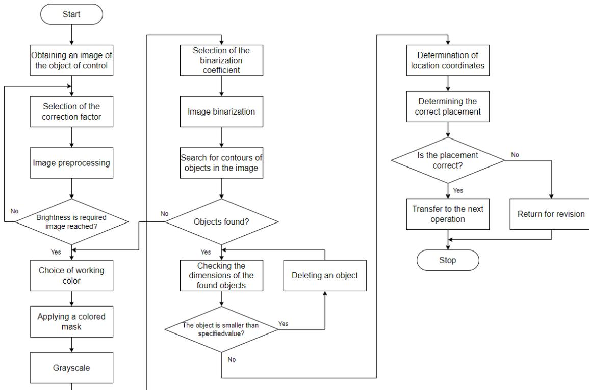
**Figure 4.** The algorithm of the automated determination system of the correct location of components on the mounting base
