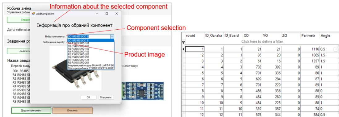
Figure 10. The screen form for adding a new component to the mounting base (left) and an example of filling in the table with the characteristics of the components (right)
