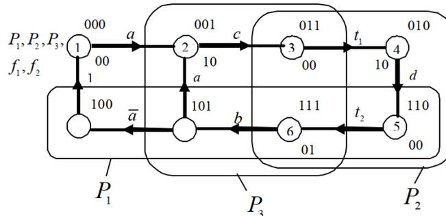
Figure 3. View of the generated graph of transitions for the automated control system of assembly operations
