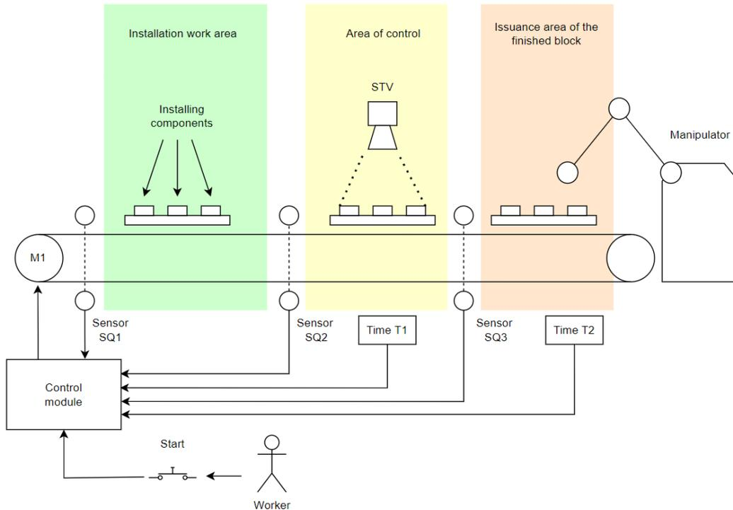
Figure 2. Scheme of industrial equipment operation for the synthesizing task the transition graph
