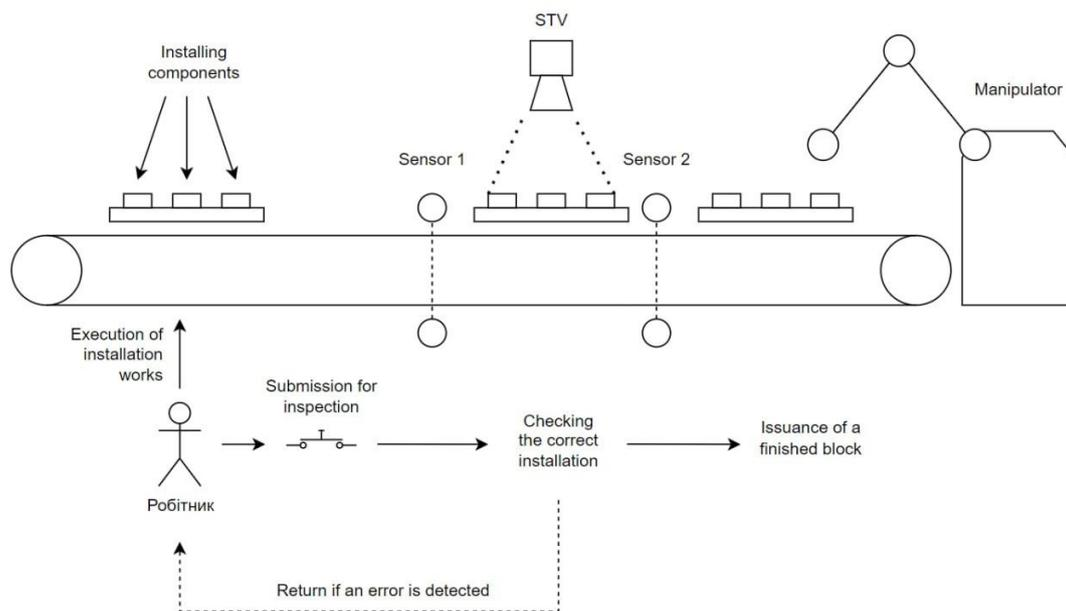
**Figure 1.** Scheme of automated system operation for monitoring the assembly operations execution
